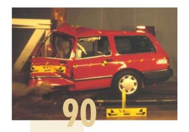
Crash test 90km/h into guard rail
